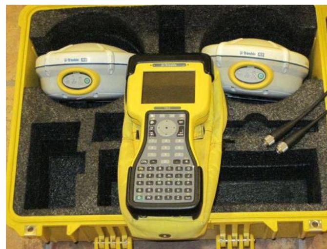
**GPS CON SISTEMA GNSS Y RTK**
